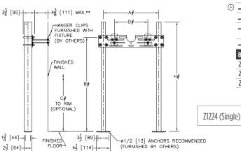
NOTES: # REFER TO ROUGH-IN GUIDE OF SPECIFIC FIXTURE FOR DIMENSION \*\* WITH STANDARD STUD LENGTH OF 6 [152]
